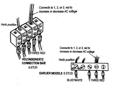
connections are generally used to increase excitation when at full amperage load the AC output of the generator falls below acceptable levels 108 volts - 60 hertz or 210 volts - 50 hertz. Note: Hertz/Speed drop is not the issue. No-load voltage may need to be adjusted when these connections are moved.
