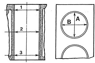
Positions for checking sleeve bore diameter
