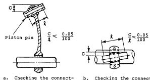
Checking the connecting rod for bend Checking the connecting rod for twist
