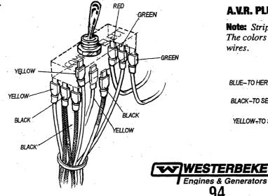
**Note:** With the selector switch in ELEC position the exciter stator windings are divided, one group is excited through the bridge rectifier and the other group through the A.V.R.
