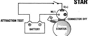
3. *Holding test.* With a battery connected to the solenoid terminal S (+) and to the starter body, manually pull out the pinion fully. The pinion must remain at that position even when released from holding with your hand.
