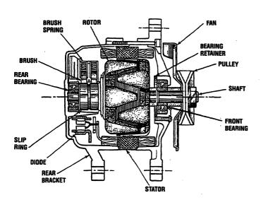
**NOTE:** The alternator connections and color coding described on the following illustrations may vary from earlier WEST-ERBEKE engines. Always refer to the wiring diagrams in this manual and also make a quick sketch of your alternator wiring before disconnecting for service.
