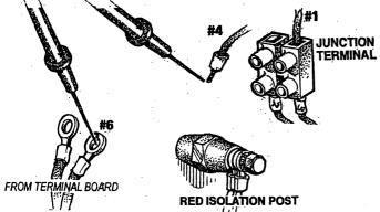
Windings Group C-2: The resistance value is measured between the lifted lead #1 from the Junction Terminal or Red Isolation Post below the transformer and lead #3 lifted off the AC Terminal Block. To totally isolate this winding group. Lift lead #2 off the terminal Block.
