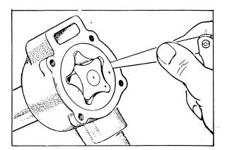
Checking rotor-to-body clearance
