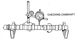
CHECKING CAMSHAFT RUNOUT.
