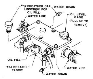
each V-drive for extra lubrication and break-in. It provides protection against scoring or galling of gears, bearings and other moving parts. Additional Molykote after break-in is not required. Reinstall the breather cap. The oil level should be rechecked after the unit has been run and allowed to sit for about a minute. Add oil if necessary.
