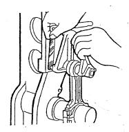
Check the connecting rod bearings for peeling, burning, melting. Replace if faulty.
