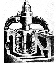
Removing ridge with ridge reamer
