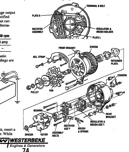
An alternate method for removing the stator winding, brush holder regulator unit and the I.C. diode rectifier assembly from the rear bracket. With the front bracket and rotor assembly separated from the rear half of the alternator:
