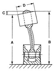
Checking connecting rod on surface plate
