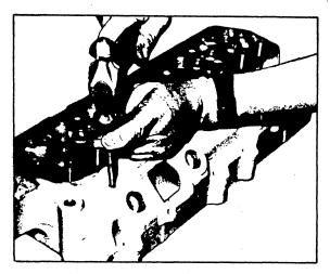
Removing precombustion chamber jet
