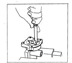
Checking rotor-to-rotor clearance
