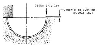
Connecting rod bearing crush
