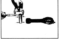
Use a micrometer to measure piston pin bushing and piston pin
