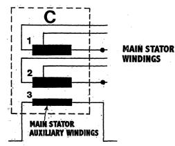
**Continuity Test:** No continuity should be found between the lifted leads to the case/ground or between the connections of
