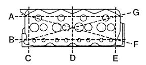
Checking cylinder head gasketed surface for flatness
