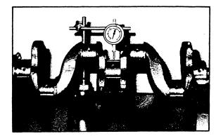
Checking crankshaft for runout
