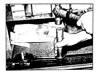
b. Heat piston on a hot plate to between 100°C and 120°C (212°F and 248°F). Install small end of connecting rod into boss and connect piston and piston pin by slowly inserting piston pin into piston.
