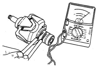
Check for continuity between the slip ring and the core. If there is continuity, it means that the coil or slip ring is grounded. Replace the rotor assembly.
