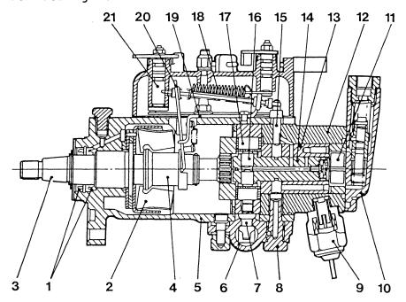
1-Drive hub seal 2-Governor weight 3-Drive shaft 4-Thrust sleeve 5-Pump housing 6-Automatic advance 7-Cam advance screw 14-Rotor
