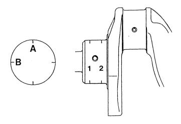
Positions for measuring journal with a micrometer
