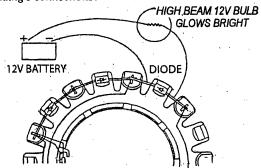
When leads are put across the diode, as illustrated, voltage passes through the diode allowing the headlight to glow brightly.
