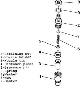
Injection Nozzle Assembly - Disassembled View
