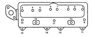
Cylinder Head Bolt Tightening Sequence
