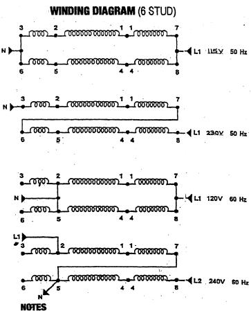
The winding diagrams show the connections necessary to obtain the correct voltage and frequency.
