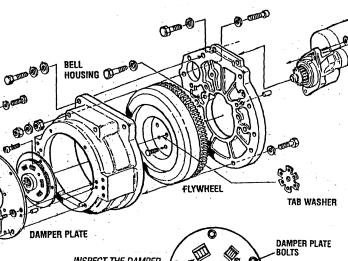
INSPECT THE DAMPER PLATE FOR WEAR AND BROKEN SPRINGS
