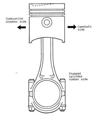
Piston and connecting rod assembly
