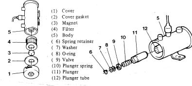
Disassembly and Reassembly of the Electric Fuel Pump for Cleaning
